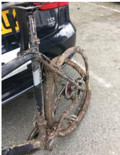
Bebbington Oval. Tubular tyres have their benefits but they must be stuck on properly to benefit properly.
