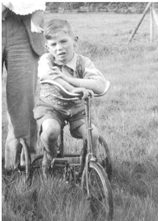
My second-hand trike on which I put many, many miles. Solid tyres (no punctures!) and a single spoon brake on the front wheel!
